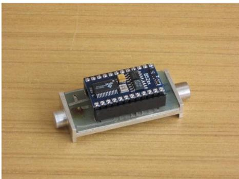
Figure 7 Control module of machine FENAUS
