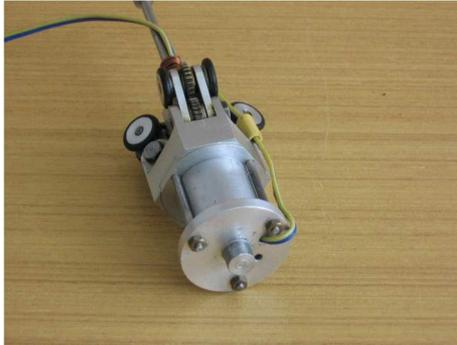
Figure 5 Drive module of machine FENAUS
