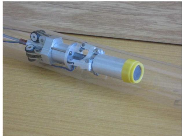
Figure 3 Modular in-pipe machine FENAUS in short version
