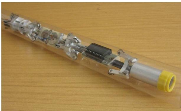
Figure 2 Modular in-pipe machine FENAUS
