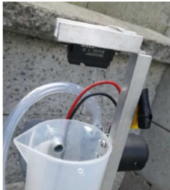
Figure 7 Distance sensor for measurement of water level
