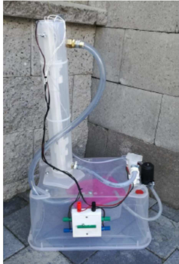
Figure 10 Realisation of functional model of water tank
