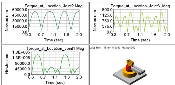
Figure 11 The graph of the torque in the joint 1, joint 2 and joint 3
