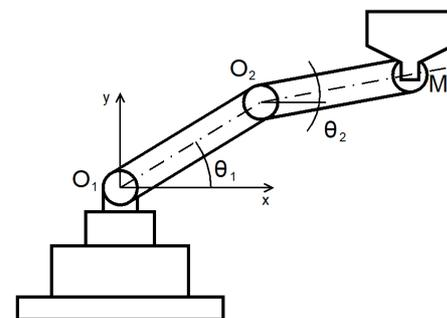
Figure 1 Model of the two link manipulator
