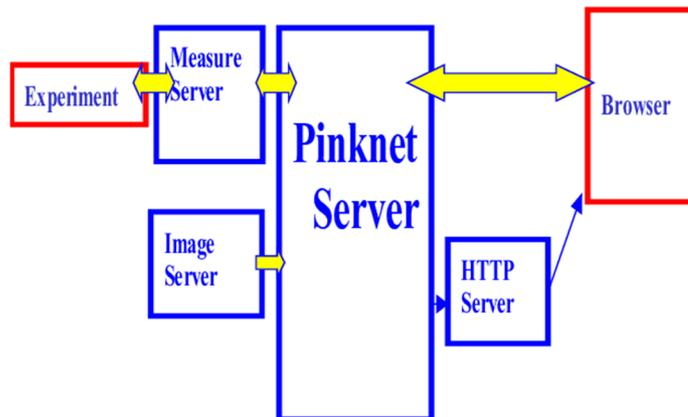
Figure 4 – Schematically representation of the remote experiment setup with Pinknet server and Image Server, Measure Server and HTTP Relay Server [9]
