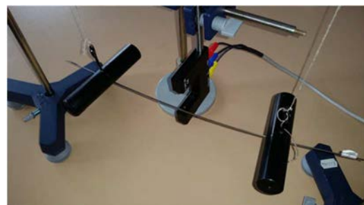
Figure 2 Experimental assembly. Vibrating wire sample crosses the infrared beam of an optical sensor (prismatic body with the shape of figure U in the centre of operation)
