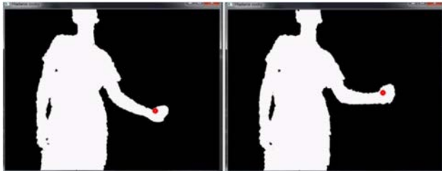
Figure 10 Scanning of the hand's movement – movement of the hand between two consequent frames.
