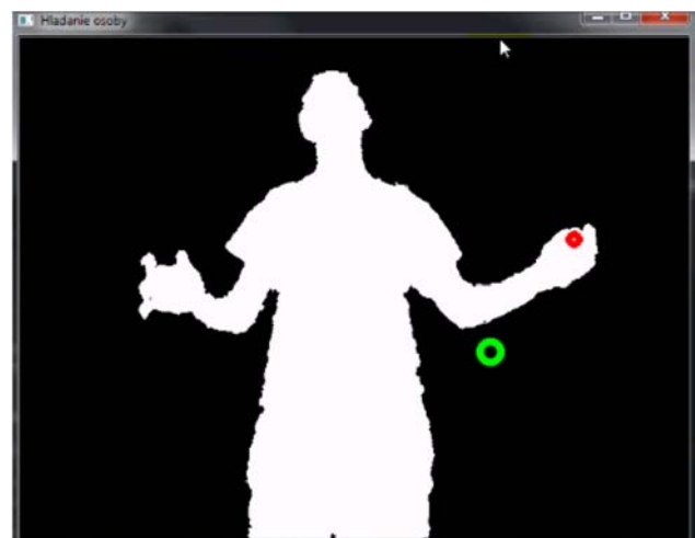
Figure 5 Skeleton identified by NiTE library. A red circle marks the right hand (human stands in front of the camera) and a green circle is the synchronization point.
