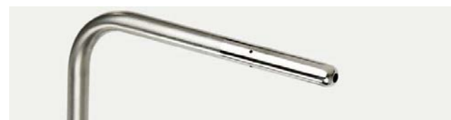
Figure 3 Prandtl tube with input and output ports.
