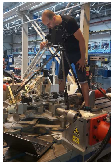
Figure 4 Drilling with positioning device and measuring of stresses with the optical device LF/Z-2
