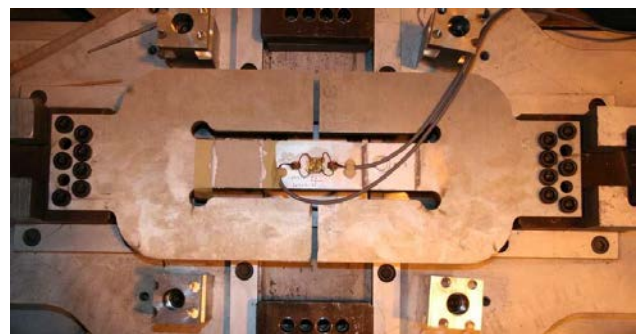
Figure 3 Aluminum sample with applied strain gauge cross
