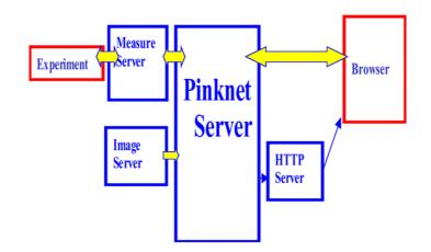
Figure 4 – Schematically representation of the remote experiment setup with Pinknet server and Image Server, Measure Server and HTTP Relay Server [9]
