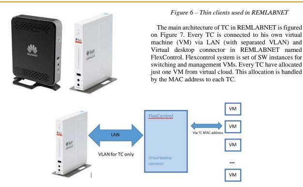
Figure 7 – Architecture of TC in REMLABNET
