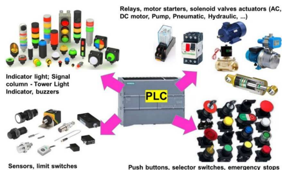
Figure 1 PLC in conjunction with sensors, switches, actuators, controls and output modules
