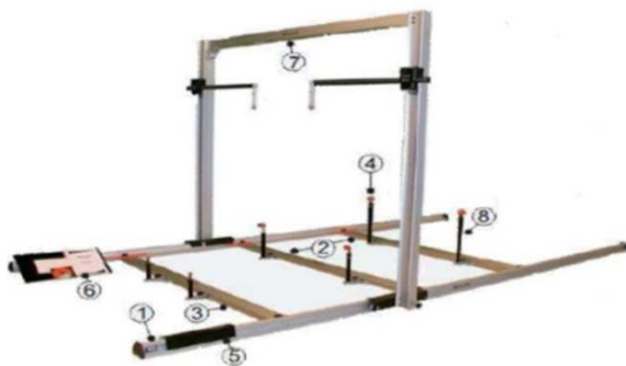
Figure 5 Mechanical device made by Autorobot, used in bodywork repairs. 1 – longitudinal beams, 2 – symmetrical
